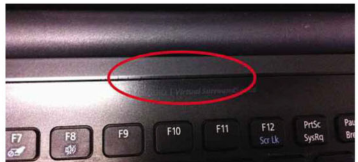
Gently pry the keyboard up from the unit using a thin screwdriver or other tool, and then slowly lift it up
